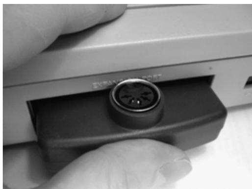
Make sure the cartridge terminals slide into the connector inside the expansion port when inserting the cartridge. Then gently apply a little more pressure on the cartridge's top side so it fully connects into the female connector inside the expansion port and sits tightly. Push it into the port until the MIDI input connector touches the C64's outer wall (where the *Expansion Port* text goes).
