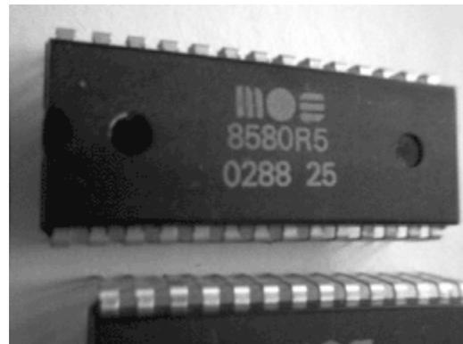
The 6581s have a printing on the top saying *6581*. *R3* or *R4* means Revision 3 or Revision 4. On the left picture above, the SID in question is a 6581 Revision 4 (good!). The right picture shows an 8580 which is always revision 5.
