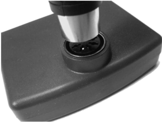
To use the MIDI interface, connect a MIDI cable from the MIDI output of your master sequencer or keyboard into the MIDI input on the MSSIAH Cartridge's top side. Read the manual for each MSSIAH application to learn how to utilize the MIDI features properly.
