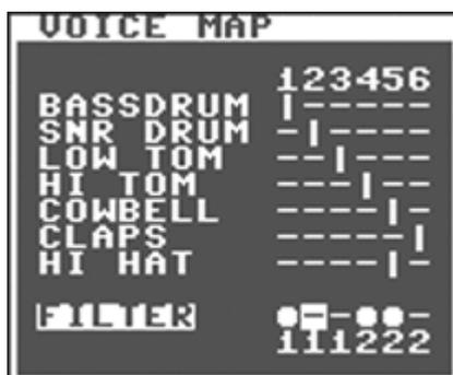
Use the **SPACE** key to toggle the filter on/off for each voice. The number in the bottom indicates which SID the voice belongs to.
