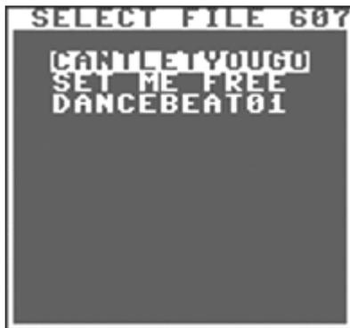
The file operations for the floppy drive make use of the operating system's basic disk functionality. There are no delete-functions and no replace-and-save options built in. If you try to save the file onto disk using an existing name the save is interrupted and the drive light flashes.
